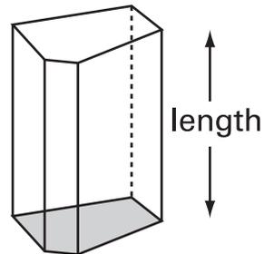
$$\text{Volume} = \text{area of cross-section} \times \text{length}$$
